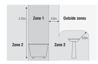
This product is suitable for use in Zone 1, Zone 2 and outside Zones in a bathroom. See diagram. If this unit is being fitted in a room containing a bath or shower, a 30mA RCD must be used - in accordance with IEE regulations.
