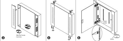
Remove the mirror panels either side of the door by removing the 4 screws (two on the top and bottom of the product).
