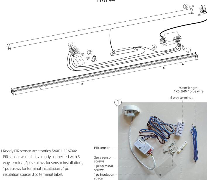
2.Exit all the wires from current terminal and LED driver (the lamp which you need to update to PIR ), take away terminal and insulation spacer,keep the driver wire.
